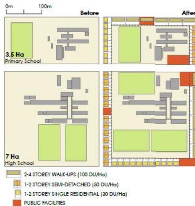
FIGURE 4.17: HOW EXISTING SCHOOL SITES CAN BE ‘WRAPPED’ WITH DIFFERENT HOUSING TYPOLOGIES TO PROVIDE PASSIVE SURVEILLANCE, OPTIMISE LAND USE AND INCLUDE OTHER PUBLIC FACILITIES (WCG, 2015)
